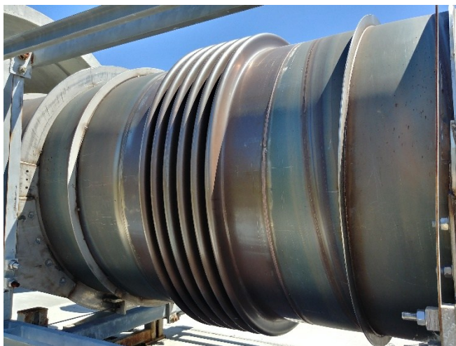
Figure 19: Metal bellows expansion joint and reinforcement ribs on display at the LIGO facility in Washington.
