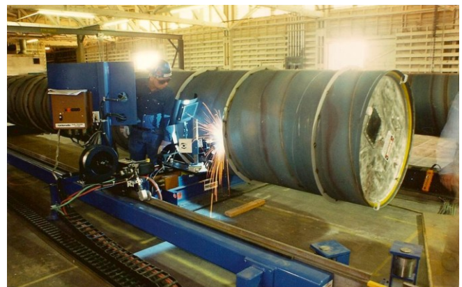
Figure 18: A segment of LIGO’s beam tube being assembled. Support rings are welded to the spiral-welded tube to increase the structural integrity of the 3 mm thick steel. (Credit: Caltech/MIT/LIGO Lab)
