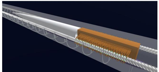
Figure 3: A launched vehicle (white) being accelerated by an adaptive nut (orange) that couples to the variable pitch screws.
