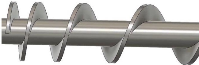
Figure 15: Example of a variable pitch screw[21].
